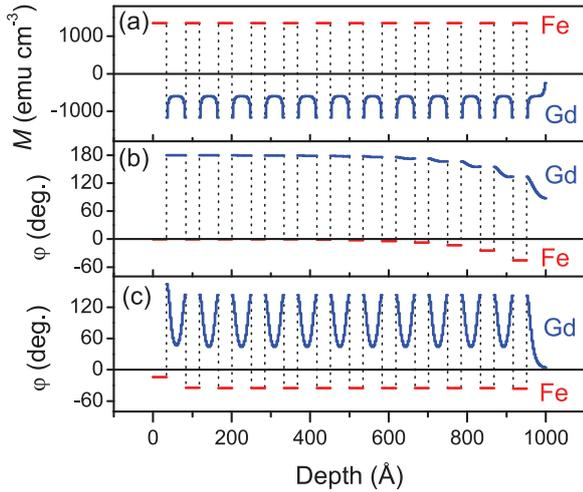
**Figure 3.** Calculated magnetization profiles at  $T = 140$  K for different magnetic fields: (a)  $H = 0.1$  kOe corresponding to Fe-aligned state (magnetization component along the magnetic field is shown), (b)  $H = 1$  kOe corresponding to surface twist state and (c)  $H = 10$  kOe corresponding to twisted state (the angle between the magnetization vector and the magnetic field is shown).
