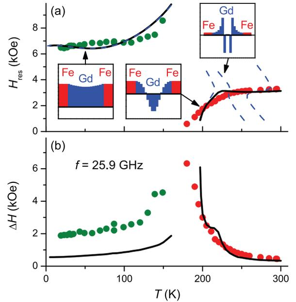
**Figure 6.** Resonance field (a) and linewidth (b) as a function of temperature at  $f = 25.9$  GHz. Points are the experimental data, lines are the result of modelling. Dashed lines correspond to the case when only local Gilbert damping is taken into account. For solid lines, the additional non-local diffusion-type dissipative term in LLE is considered. Insets show calculated precession profiles (real part of eigenvectors) for different modes normalized on static magnetization distribution.
