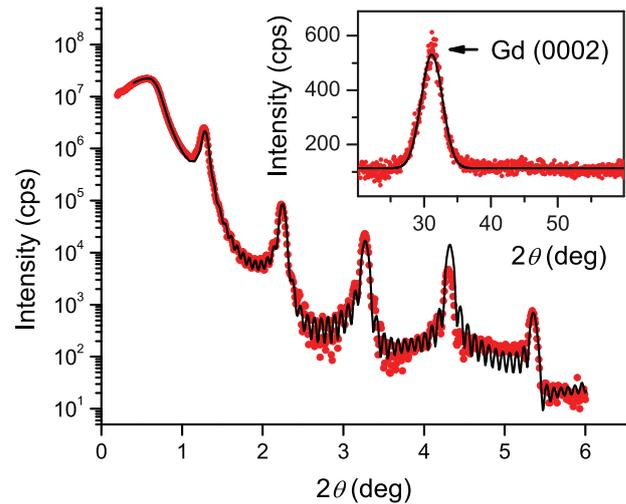
**Figure 1.** Experimental XRR spectrum of the studied glass/Cr(50 Å)/[Fe(35 Å)/Gd(50 Å)]<sub>12</sub>/Cr(30 Å) multilayer structure (points) and its approximation (line) with parameters shown in table 1. The inset demonstrates the experimental XRD spectrum.
