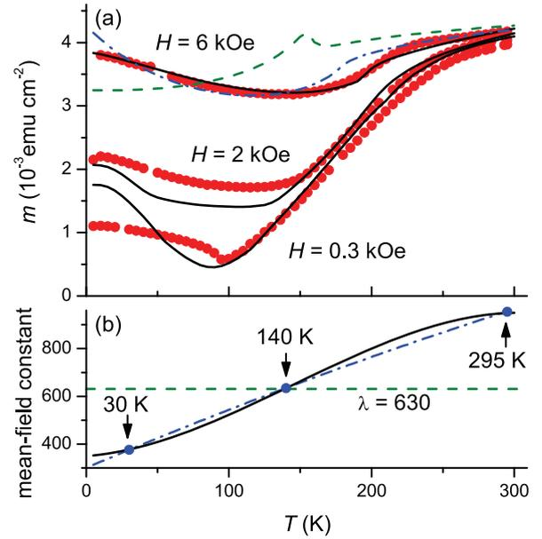
**Figure 4.** Magnetic moment per unit area as a function of temperature measured at  $H = 0.3, 2$  and  $6$  kOe (a). Points are the experimental data, lines are theoretical calculations with different  $\lambda(T)$  dependences (b). The dashed line corresponds to constant  $\lambda$ , the dash-dotted and solid lines correspond to the second- and third-order curves  $\lambda(T)$  respectively.
