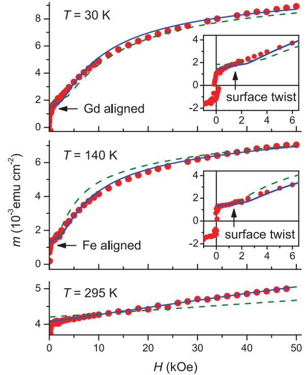
**Figure 2.** Magnetization curves at  $T = 30, 140$  and  $295$  K. Points are the experimental data, dashed lines correspond to their best fit with constant  $\lambda$ , solid lines correspond to the best fit with temperature dependent  $\lambda$  (see table 2). Insets show low field regions with hysteresis loops.
