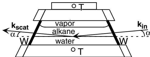
FIG. 1. Cross-sectional view of sample cell:  $W$ , Mylar windows;  $T$ , thermistors to measure temperature. The kinematics of surface x-ray reflectivity is also indicated:  $\mathbf{k}_{\text{in}}$  is the incoming x-ray wave vector,  $\mathbf{k}_{\text{scat}}$  is the scattered wave vector, and  $\alpha$  is the angle of incidence and reflection.
