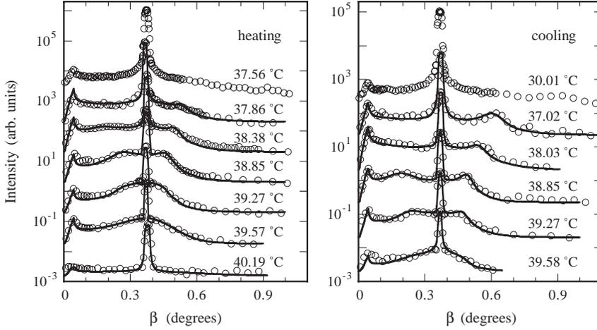
Fig. 3 – Transverse diffuse scattering ( $\beta$  scans) for a heating-cooling cycle (heated first, then cooled); lines are fits described in the text. Curves are shifted for clarity.
