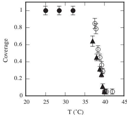
Fig. 5 – Interfacial coverage (fraction of interface covered by the low-temperature solid phase) as a function of temperature. Open circles: heating curve; filled triangles: cooling curve; dots: from earlier reflectivity measurements.
