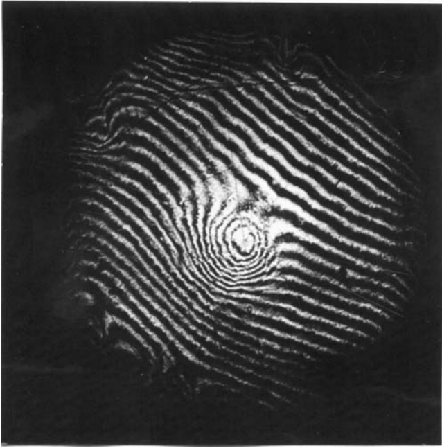
FIG. 16. Interference pattern of a charged interface between liquid and solid ^4\text{He} . Here the electrons are concentrated in the central region to enhance the visibility of the deformation. The parallel fringe pattern outside the center results from a small angle between the two interferometer plates. The field of vision is about 2 cm in diameter. From Savignac and Leiderer, 1982.
