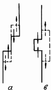
Fig. 2. Possible types of kink collisions: (a) the "normal" collision; (b) the collision with a "jump" in the next row.
