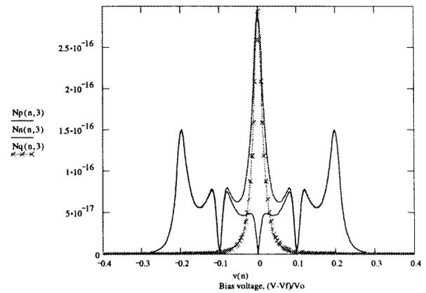
**Figure 3.** Recovered spectrum  $N_q = N_p(v) - |N_n(v)|$  (crosses), sum  $N_p = N_e(v + v_{if}) + N_e(v - v_{if})$  (full curve) and difference  $N_n = N_e(v + v_{if}) - N_e(v - v_{if})$  (broken curve) of output signal shifted dependences  $N_e(v + v_{if})$  and  $N_e(v - v_{if})$ .
