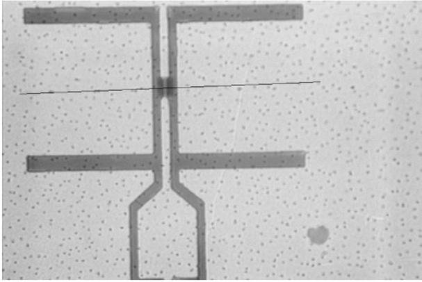
**Figure 1.** The layout of integrated structure with a bicrystal Josephson junction and a double-slot antenna. The horizontal line in the centre indicates the bicrystal grain boundary. A resistive low-inductive shunt made of Au wire 0.03 mm thick is bonded to the contact pads outside the view.
