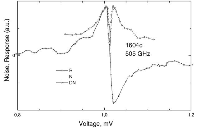
**Figure 2.** Selective detector response  $R$  and noise  $DN$ , the latter after the deduction of autonomous noise and extraction of the square root.
