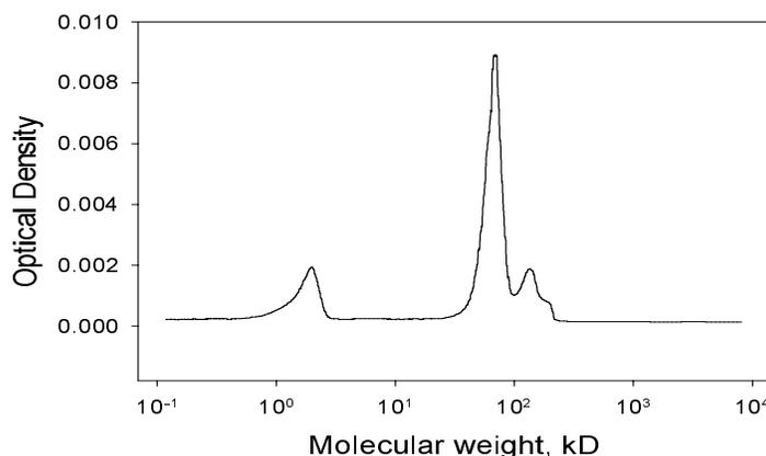
Figure 3: High-performance liquid chromatogram of the BSA compound; the column is TSK G2000 SW Spherogel,  $10\ \mu\text{m}$ ,  $7.5 \times 600\ \text{mm}$  (LKB); the solvent current rate is  $0.5\ \text{ml/min}$ .
