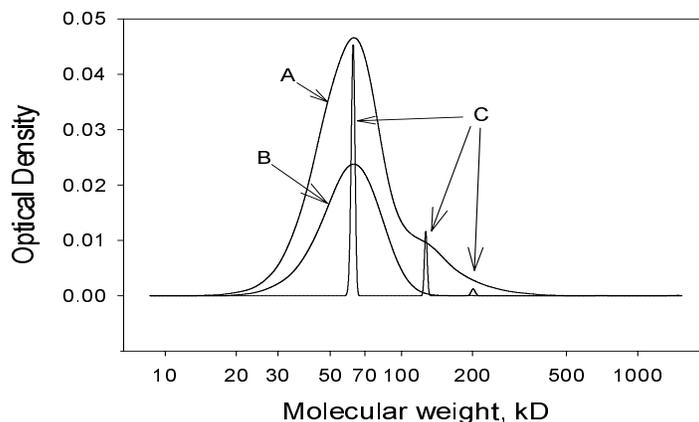
Figure 2: The use of the RECOVERY software package for the initial data given in Fig.1: (A) the BSA chromatogram obtained for a TSK-gel column; (B) point-spread function (BSA monomer chromatogram); (C) recovering result of the chromatographic separation data with the use of the `Dconv2_` program from the RECOVERY software package.
